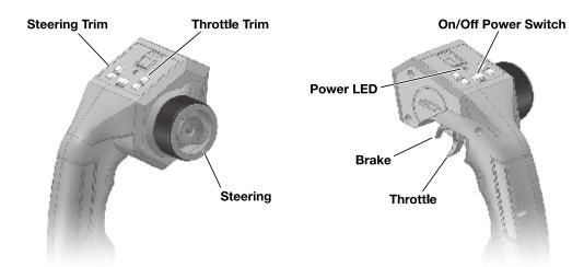
Slide the power switch to turn the TX on. The "POWER" LED should illuminate. If not, turn off the TX and check the batteries to make sure each cell is firmly in place and in the proper direction. If the TX LED blinks, the batteries are low on power and should be replaced.
